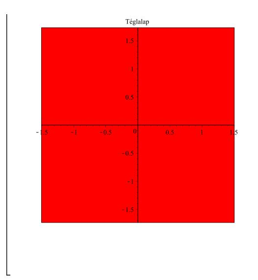
We also have to mention the **polygonplot** procedure from the **plots** package. It waits as a first parameter for a list of two-element lists the way we prepared that in the variable *T*. Each of the two-element lists describes the coordinates of a vertex of the polygon to be drawn. The other parameters are the usual options of the **plot** procedure.
