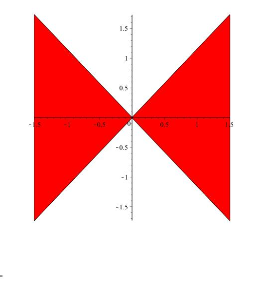
The graph has become a little bit crisscrossed although we did nothing else but to exchange the two middle elements of the T list. The **polygonplot** supposes that the two-element lists which are next to each other in the list are the coordinates of adjacent vertices thus it connects these with a line. It matters, therefore, in which order the vertices of the polygon to be visualized are written down.
